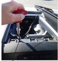
Screws to remove radio bezel
