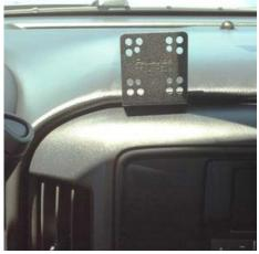
InDash installed showing Left mounting location
